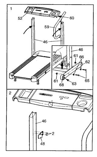
3. Cut the plastic tie holding the cage nut in the upper end of the Left Handrail (45).
